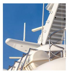
OMNI-600 (or OMNI-402), mounted using the provided 316 Stainless Steel L-bracket
